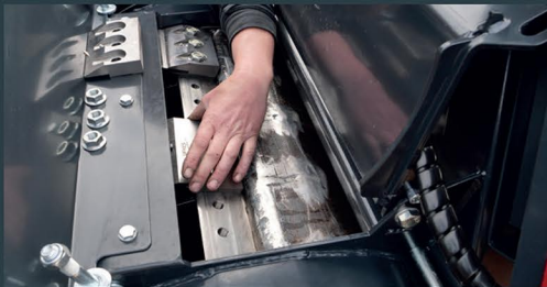
Standard equipped with quick change knives
